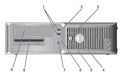
1 USB 2.0 connectors (2) Use the USB connectors on the front of the computer for devices that you connect occasionally, such as joysticks or cameras, or for bootable USB devices (see your online *User's Guide* for more information about booting to a USB device).
