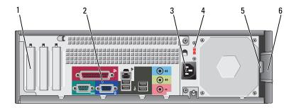
1 card slots Access connectors for any installed PCI and PCI Express Cards.
